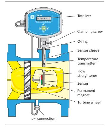
equation of state together with the corresponding standard conditions. Then this values is summed up in the standard volume totalizer and stored in the data logger.
